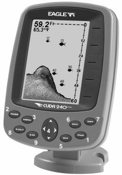
Eagle Cuda 240 Sonar, front view, showing screen and keyboard. (A close-up of the keyboard can be found at the beginning of Sec. 6)
